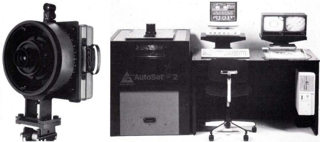
Figure 2.15: CRC-1 camera (left) and AutoSet-2 (right) as components of the STARS system used in industrial photogrammetry.
