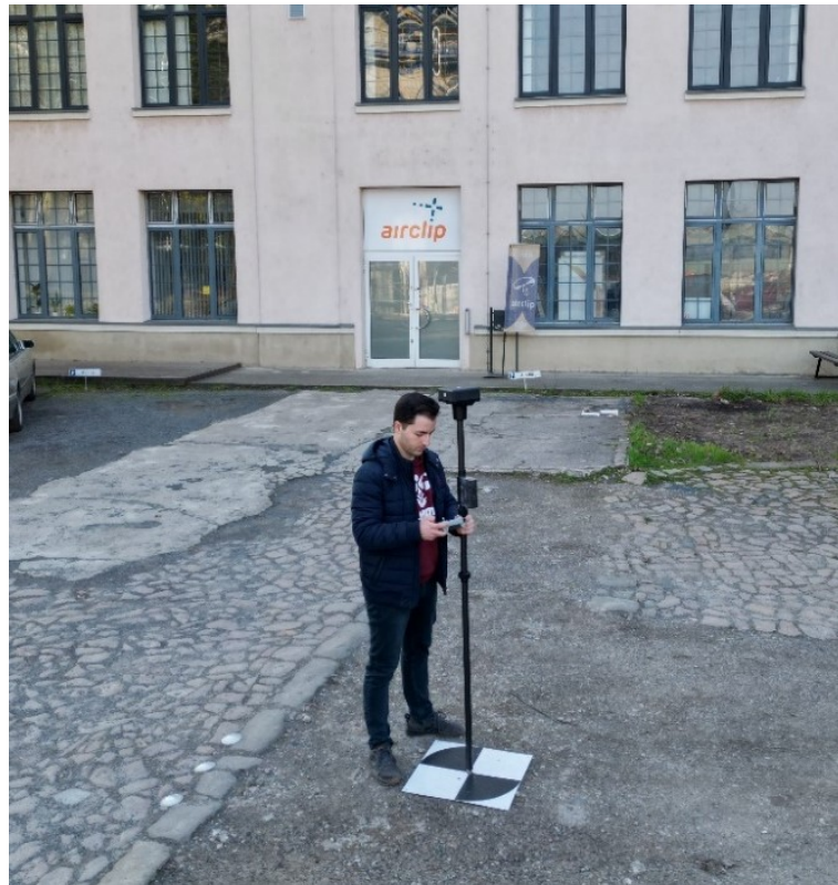
Figure 5.14: Photograph from the GCP coordinate measurement stage.
