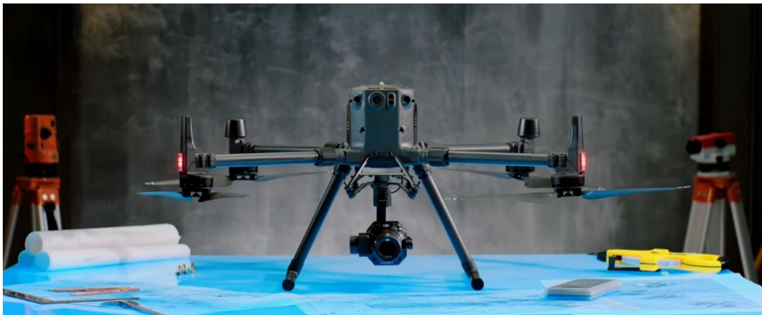
Figure 5.8: DJI Matrice 300 RTK and Zenmuse P1.
