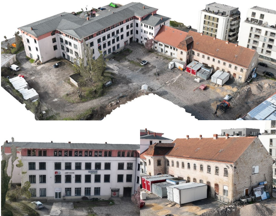
Figure 6.2: 3D model created from photographs captured by DJI Mavic 3E.
