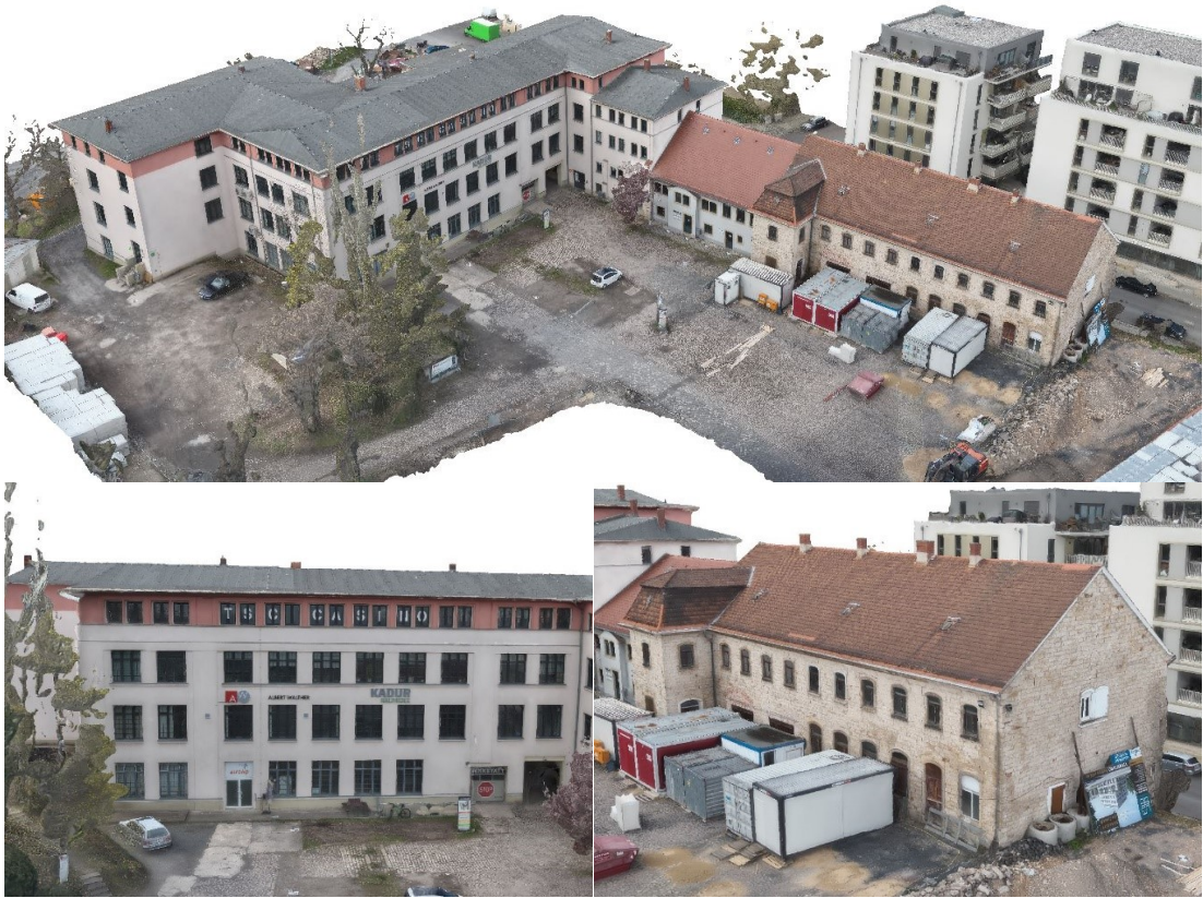
Figure 6.3: 3D model created from rgb photographs captured by DJI Mavic 3T.
