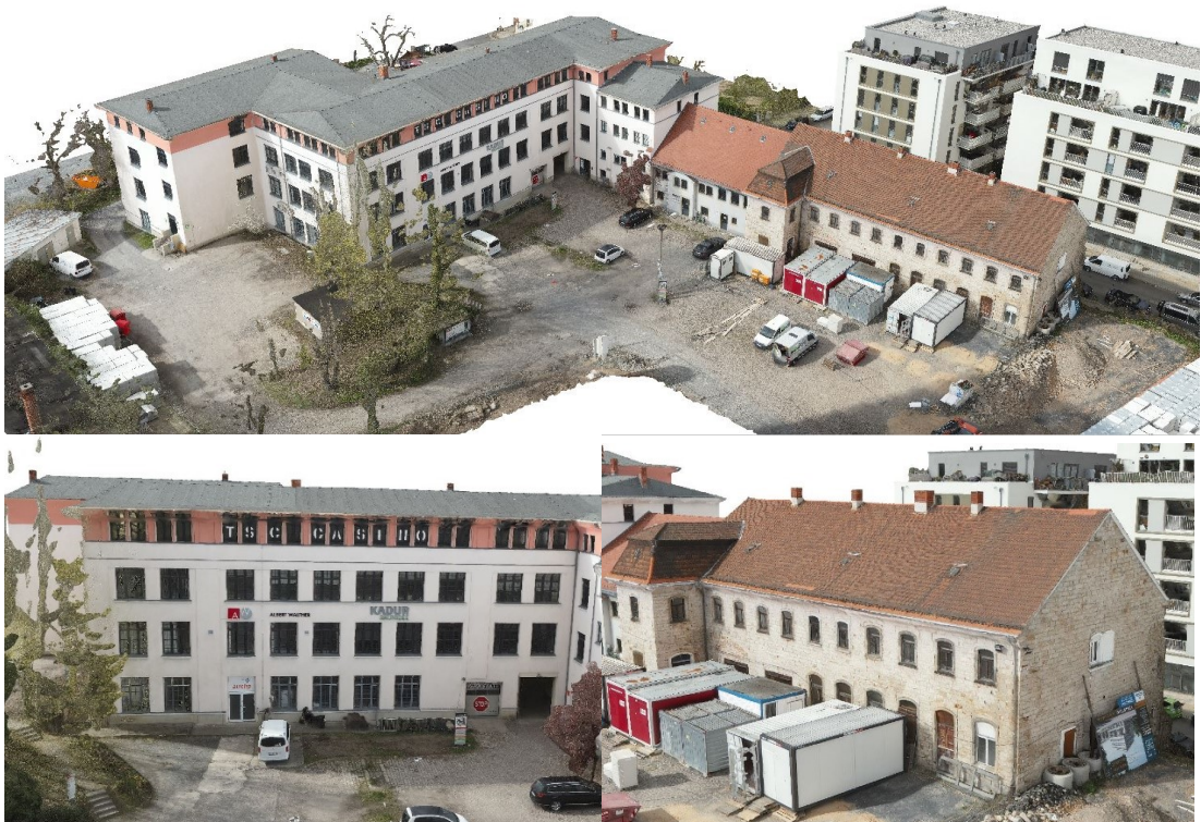
Figure 6.8: 3D model created from photographs captured by DJI Matrice 300RTK.
