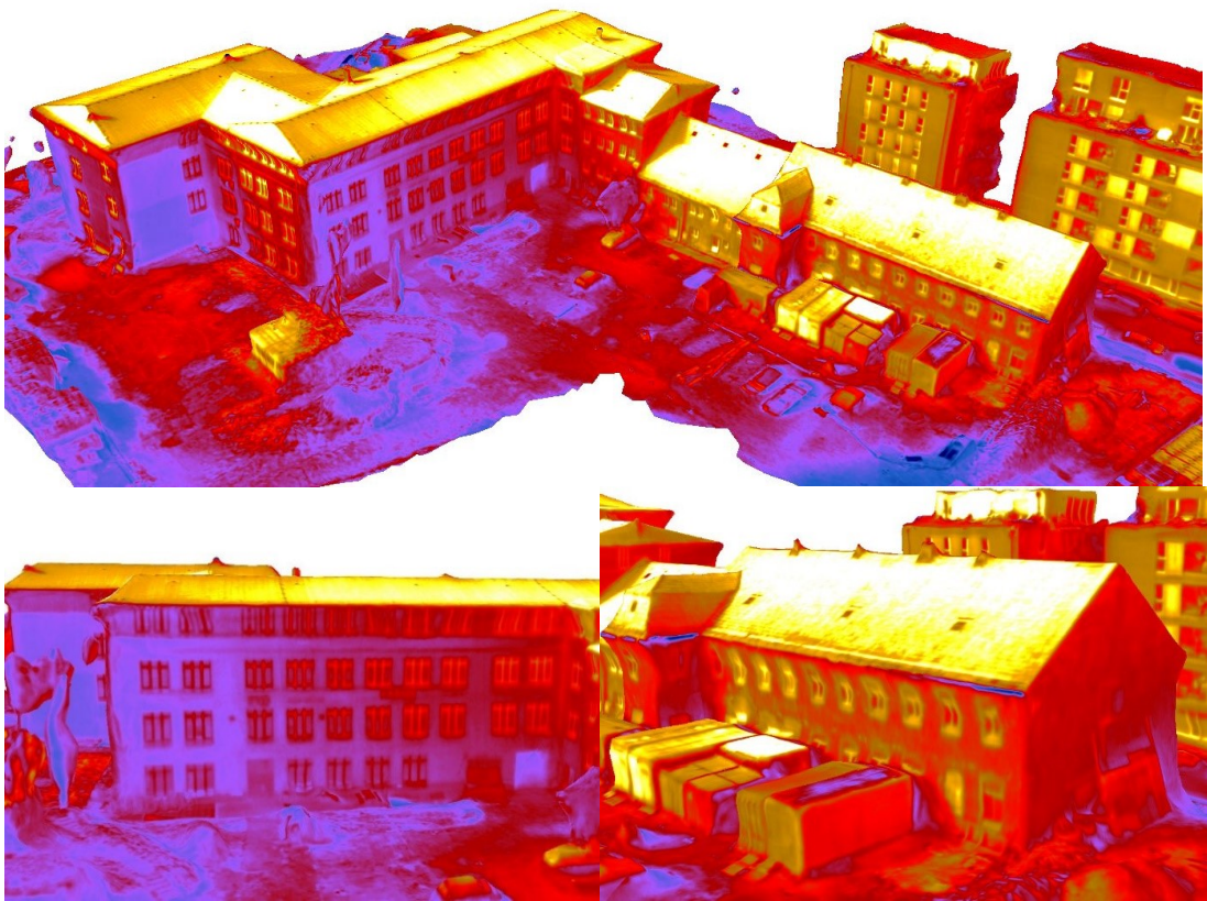
Figure 6.7: 3D model created from thermal photographs captured by DJI Matrice 30T.
