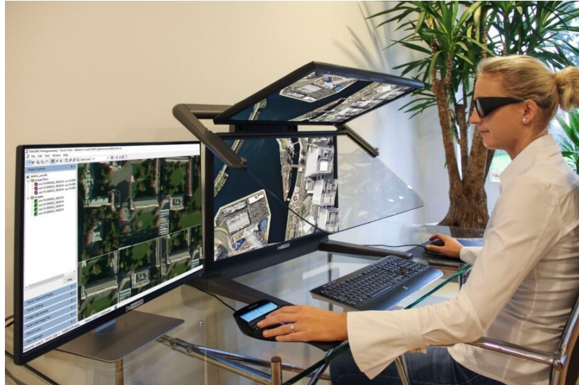
Figure 2.23: A setup for digital photogrammetric stereoplotting.
