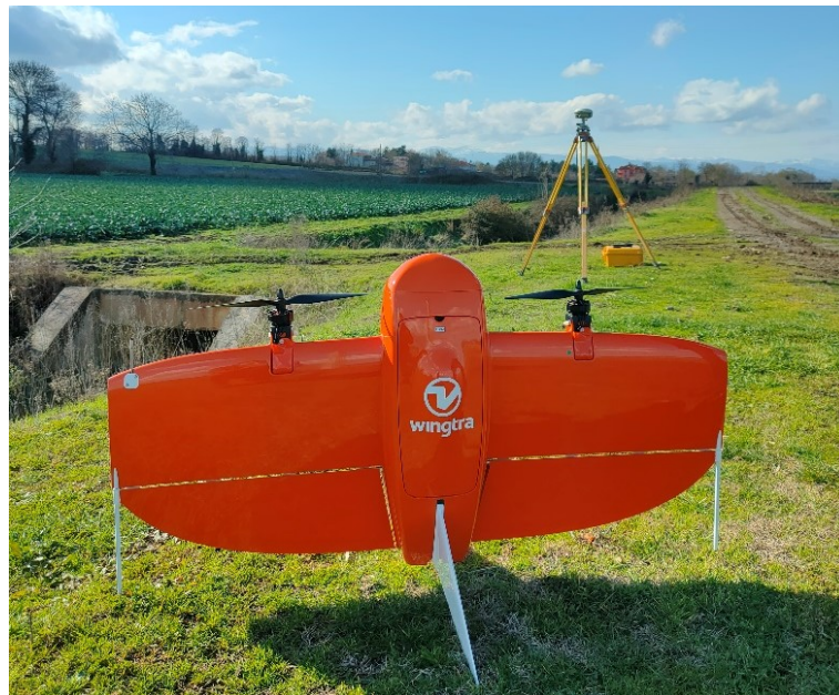
Figure 5.10: WingtraOne fixed wing, VTOL UAV
