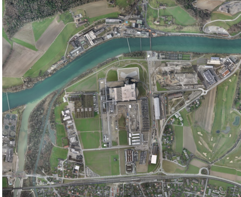
Figure 2.5: An orhomosaic sample created from 452 aerial orthophotos via WingtraOne fixed wing UAV
