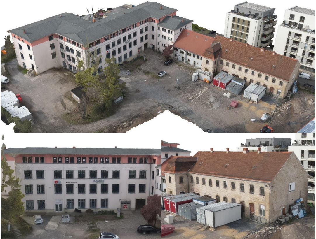
Figure 6.6: 3D model created from rgb photographs captured by DJI Matrice 30T.
