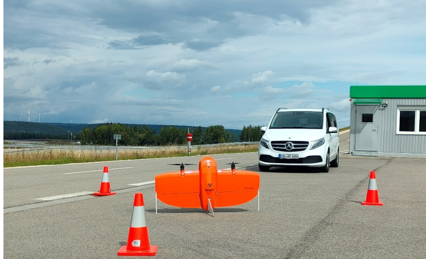
Figure 3.5: WingtraOne as an example of fixed-wing UAV.
