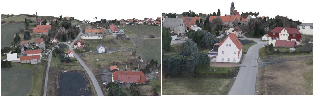
Figure 6.9: 3D model created from photographs captured by WingtraOne Gen II.
