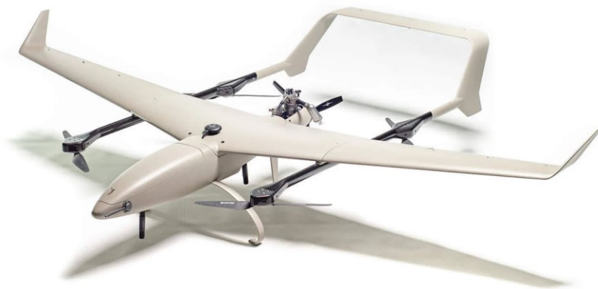
Figure 3.6: Alti Reach fixed-wing UAV which has a liquid fuel engine and VTOL feature.
