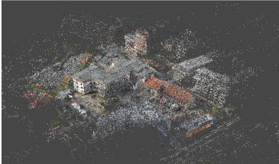
Figure 5.20: Present the output tie point formed by the data captured with DJI Mavic 3E.
