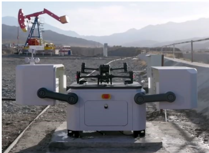
Figure 5.7: DJI Matrice 30 T landed on the DJI Dock Station.
