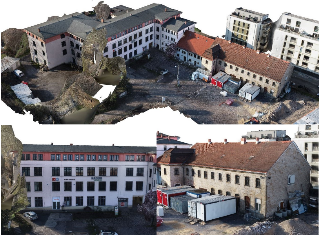
Figure 6.5: 3D model created from photographs captured by DJI Phantom 4 RTK.
