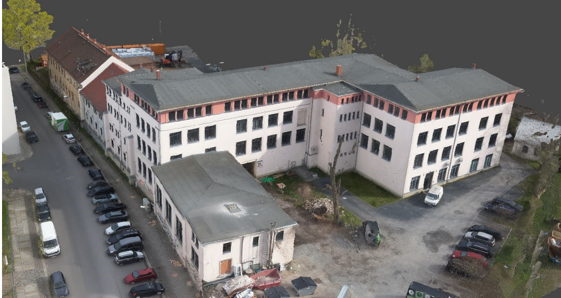
Figure 5.27: Output textured mesh created from the data captured by the rgb camera of DJI M30T.
