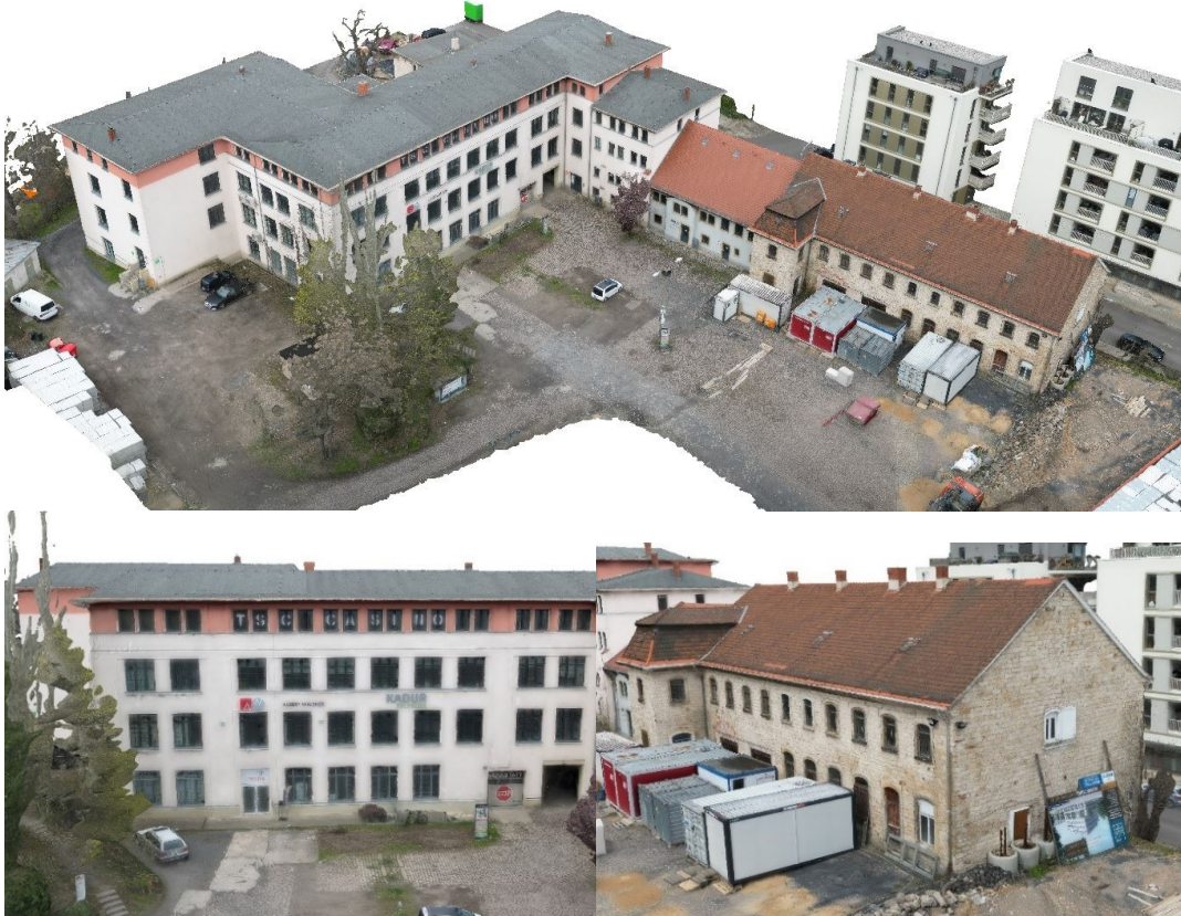
Figure 6.1: 3D model created from photographs captured by DJI Mini 3 Pro.
